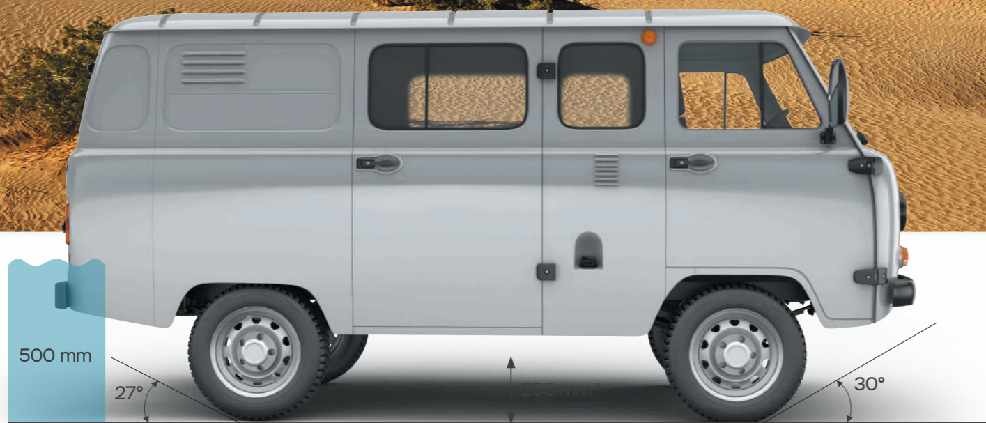
Minimum height of the chassis - distance from the ground to the axle housing.
